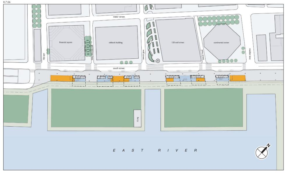
roadway (one in each direction). The buildings would be constructed through the middle of the roadway, requiring a reconfiguration of the roadway structure. The lobbies for the building would be located below the FDR viaduct. Pavilions could still be constructed beneath the FDR Drive north of the Brooklyn Bridge. The potential building scenarios are detailed below in Table 19-1.
